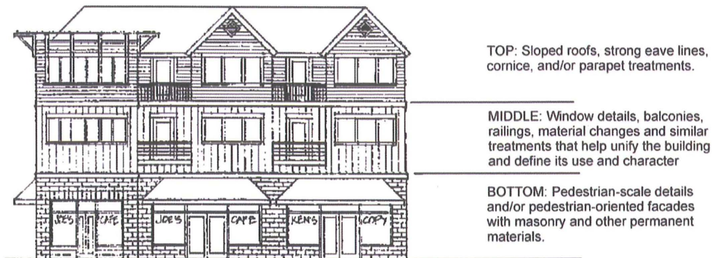
Figure 9 – Building facade with a distinct top, middle, and bottom.
