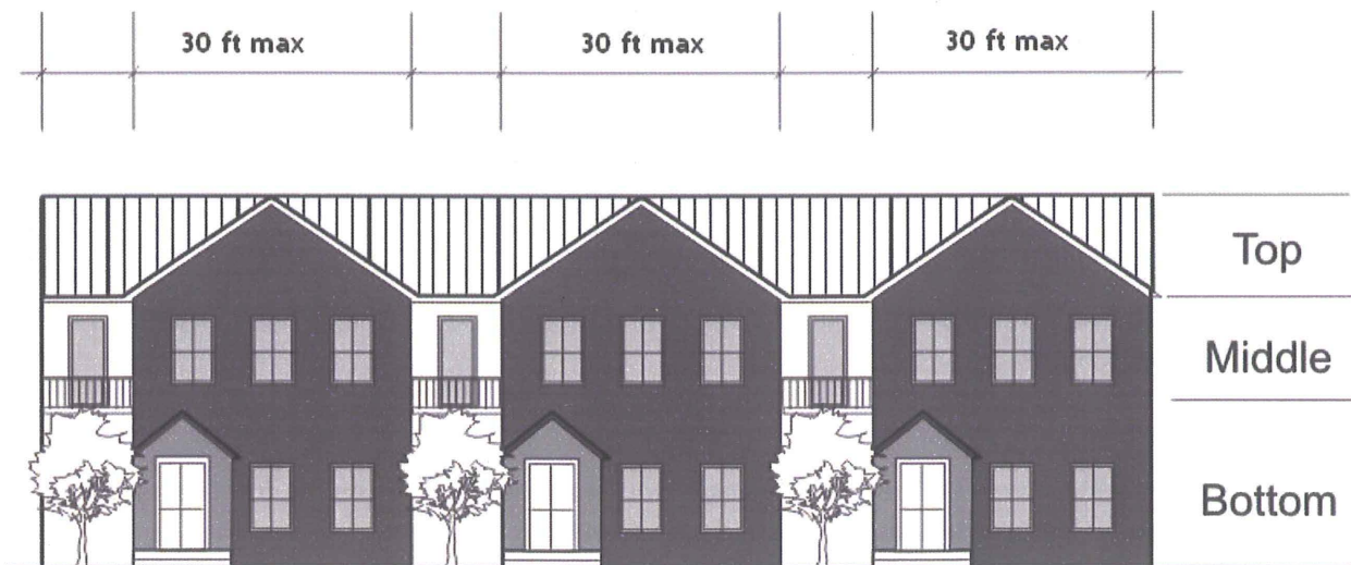
Figure 45 – Horizontal elements of a typical townhome.
