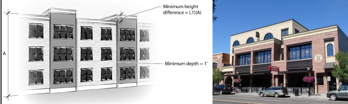
Roofline modulation examples for flat roofs.
