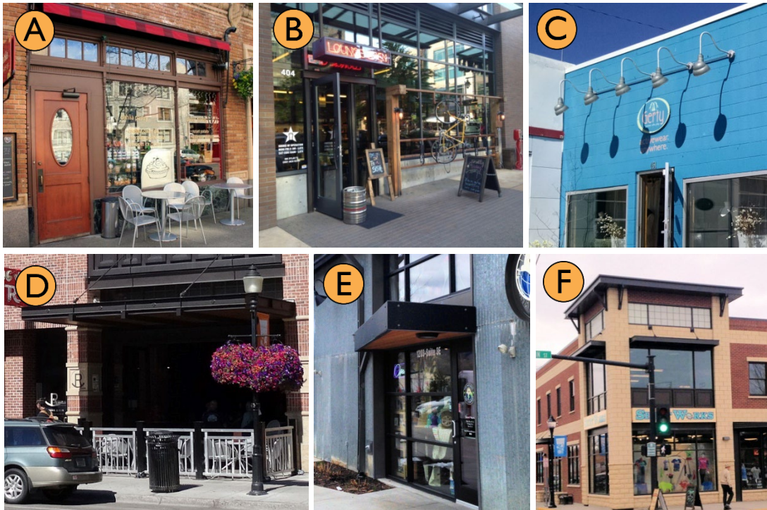
Examples of elements attached to facades that enhance the visual intrigue of the building. A = retractable awning. B = custom hanging bike rack and repair station integrated as a storefront design element. C = decorative façade/sign lighting. D and E = custom decorative canopy. F = decorative tower.
