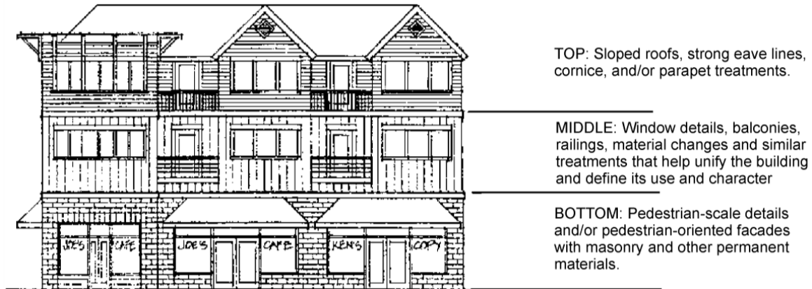
Figure 10– Building facade with a distinct top, middle, and bottom
