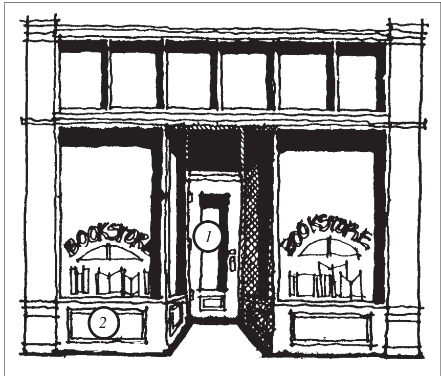
This traditional storefront sketch illustrates a (1) recessed entry and (2) kickplate.
