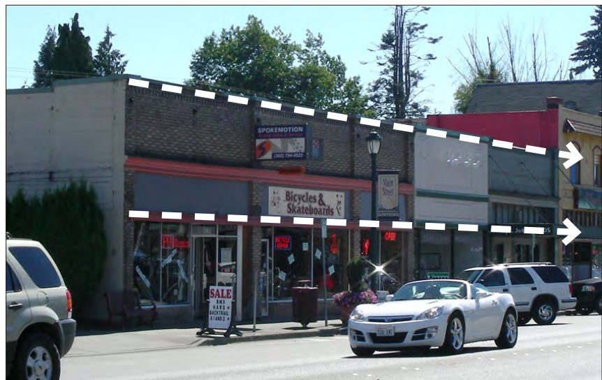
New construction should relate to existing historic structures by maintaining the alignment of horizontal features, producing a similar floor to floor height, dividing a larger facade into smaller modules and maintaining the visual scale of the building.
